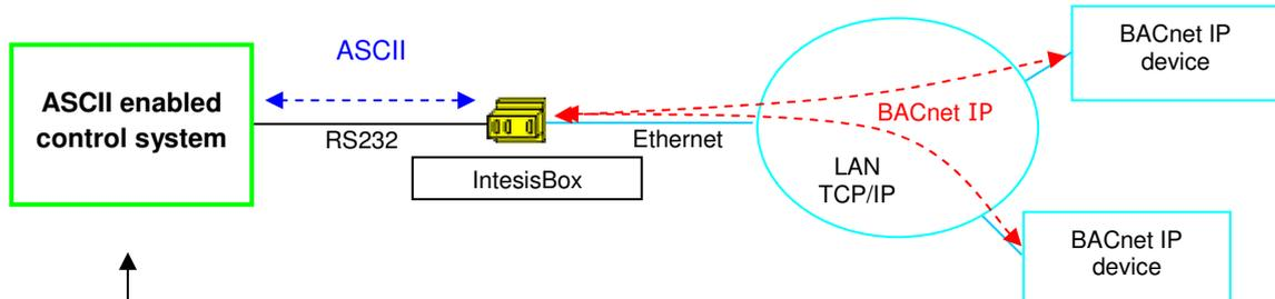
**Control system with ASCII master interface.**
