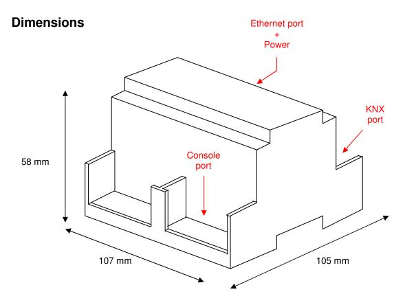
Free space recommended to install the device into a cabinet (wall or DIN rail mounting), with space enough for external connections:
