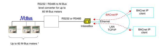
The following is a diagram of a large installation (up to 500 meters):
