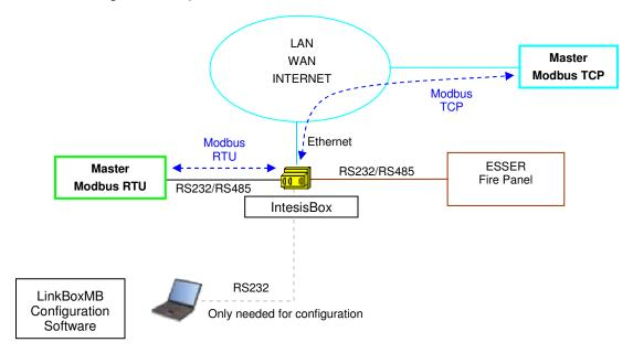
Monitor & Control your network of ESSER fire panels remotely from your Control Center using any commercial SCADA or monitoring software with Modbus TCP driver.
