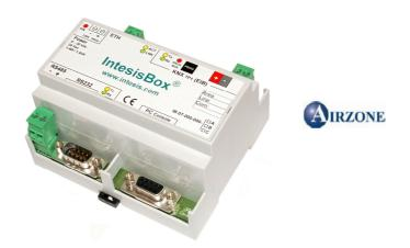
Gateway for integration of AIRZONE Innobus air conditioning into KNX EIB installations.
