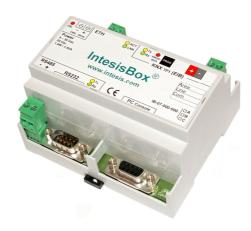
Gateway for monitoring and control KNX EIB installations from programmable controllers (AMX, Crestron, Litetouch...), touch panels, PCs... using simple text messages.
